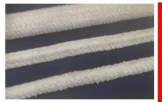
Keramab<sup>®</sup> braided packing is reinforced with glass or metal wire and contains approximately 20% organic carrier fibre to facilitate the carding process. The carrier fibre burns out at a low temperature, but this has no effect on the properties of the ceramic fibre.
